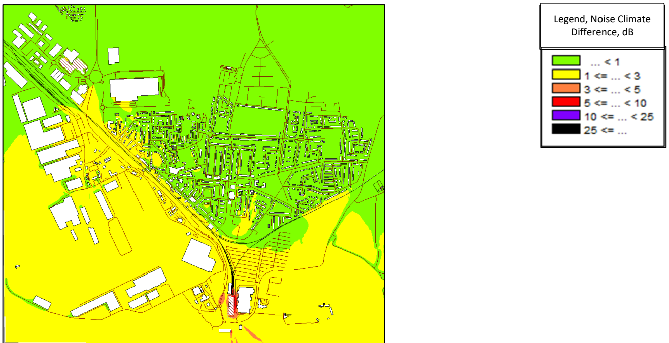
Diagram 15.4.5: Image showing the difference between the LA10,18hr (dB) noise climate during 2038 London Resort operation design day and baseline ambient noise level conditions around the Essex Project Site.
